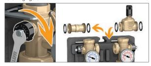
The mounting is different depending on the direction of the discharge flow:
